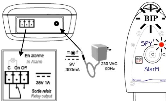
By default, the alarm is alternatively on and off 4'only for the relay.
