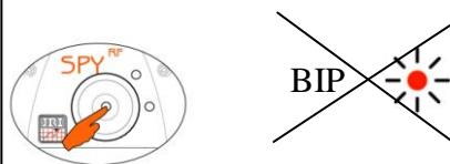
Stop is temporary (4 min) only for the relay. The alarm will go on again until it will be acknowledged by Sirius.
