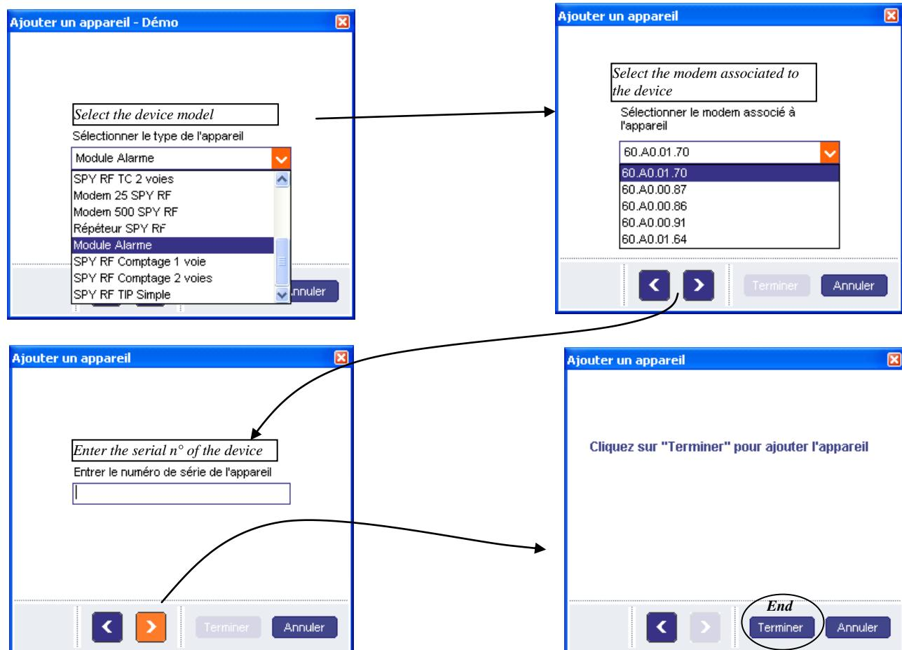
After Ending, the window will close and the Spy RF AlarM is installed and appear in the fleet
