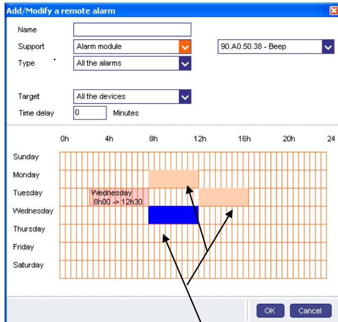
Time period in which the remote alarm is activated. Each square equals to 30 minutes. The selection or deselection of a period is done by a click / slide.
