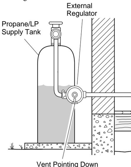
**Figure 12 - External Regulator with Vent Pointing Down**
