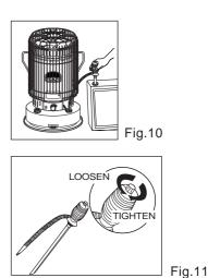
After fueling the fuel tank of the heater by using siphon pump, make sure that you loosen (counter clock wise) the cap on the siphon pump to drain
