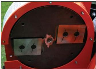
Cantilever rotor/bearing and reversible chipper blades make maintenance a simple process.
