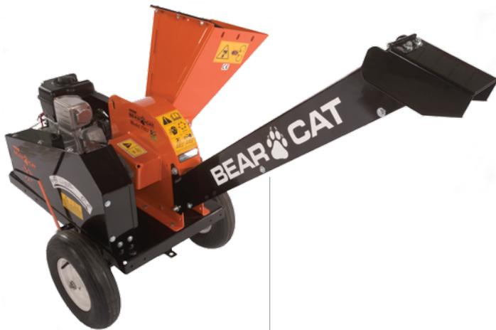
When equipped with the optional discharge chute, chips can be directed into a cart, barrel or truck bed for easy clean up (Model CH45390 with 4.5" Square Discharge Chute Accessory).
