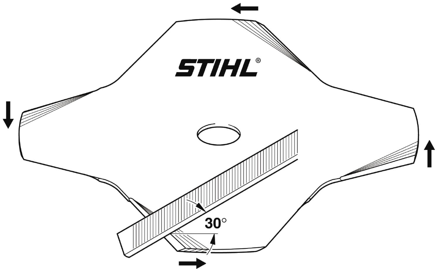
**WARNING!** Never use a bent or cracked metal cutting blade and never attempt to straighten or weld them. Such blades might shatter at high speeds and cause serious or fatal injury.
