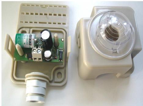
Pass the cable through the cable gland and wire to the board terminals using a flat screwdriver.
