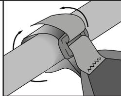
You can also move the platform forward or back slightly on the pontoons by loosening and tightening the pontoon webbing attachment straps.
