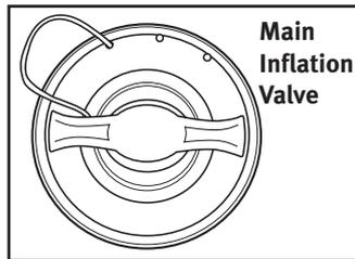
Each valve has a center button that opens and closes the valve by simply pushing down, and turning a quarter turn. The valve is open when the center button is down and closed when it is up.
