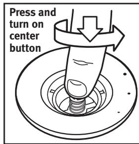
**Before inflating, make sure the valve is in the closed position.**
