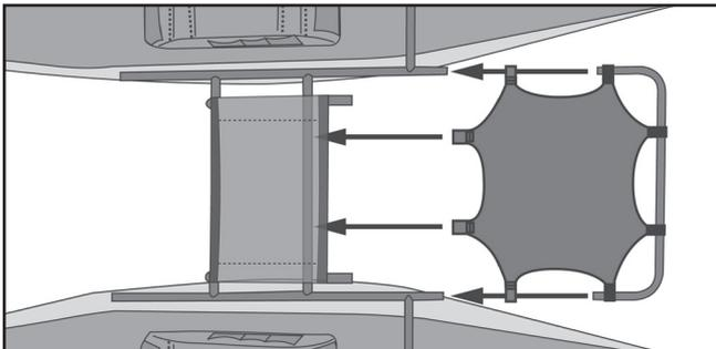
frames. Insert a short clevis frame pin on either side of the frame from the top down into the holes where the cargo deck frame slides into the
