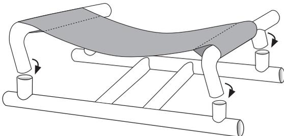
press in all four of the seat frame receptacle posts, then put your full weight evenly across both seat platform rails and press them all the way down.
