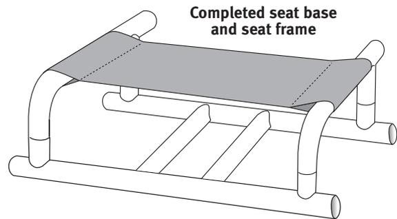
**Locate the seat base and find the curved legs. With the curved legs to the front, insert the seat platform rails onto the pontoon frame posts.** (The front of the pontoon frames are the ends labeled "L" and "R").
