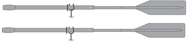
Then adjust the rubber oar stops evenly on both oars for optimum rowing position.
