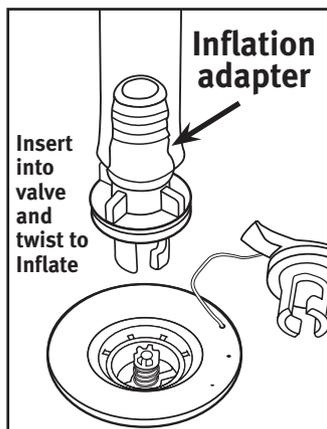
**Inflate the main chamber in the pontoon to about 3/4 full. Do not inflate beyond 3/4 full because it will make the next step very difficult—attaching the pontoons to the frame.**
