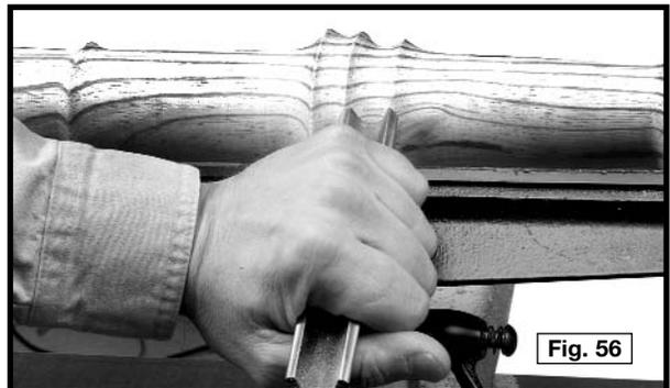
The gouge is placed on edge on the tool rest so that the grind of the chisel forms an approximate right angle with the work (Figs. 57). The chisel contacts the work at the center of the cutting edge. Hold the tool so that the centerline of the gouge is pointing directly toward the center of the revolving stock. This starting position is important to prevent the gouge from running along the surface of the work.
