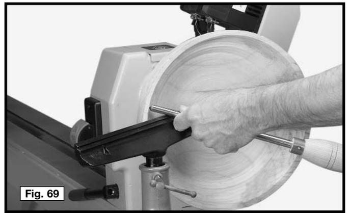
6. Use an outboard tool rest (B) Fig. 68 for all outboard turnings.
