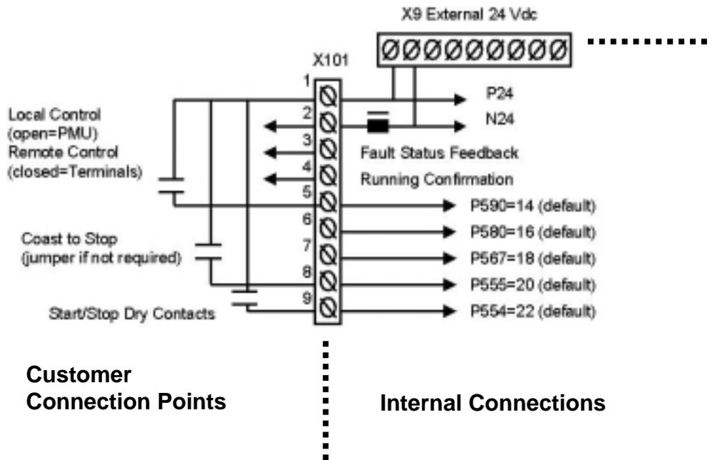
Step 1: Dry set of contacts between terminals X101, pin#1 and pin#5 for Local/Remote Mode Selection. Jumper if not required.
