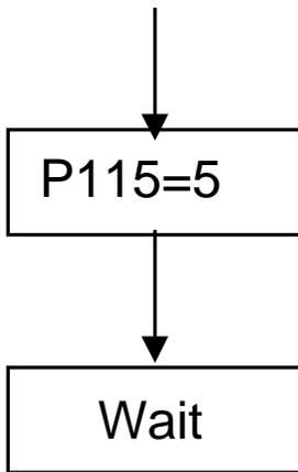
P115=5 Controller Optimization Alarm message “A080” will appear, and a start command must be issued within 20 seconds to perform the test, otherwise P115 will unset.
