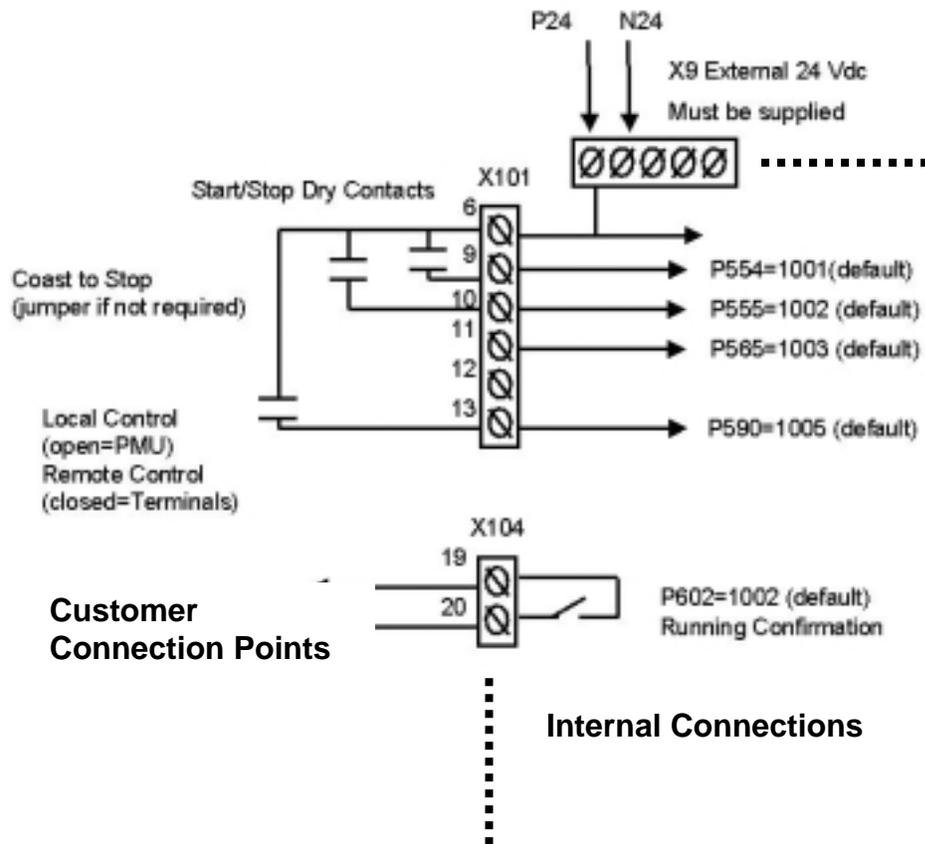
Step 1: Dry set of contacts between terminals X101, pin#6 and pin#13 for Local/Remote Mode Selection. Jumper if not required.
