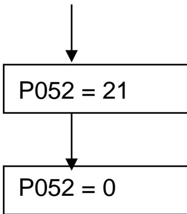
With DC BUS connected to the COMMON DC BUS of the system, set P52=21 and provide a start command at terminal X101, pin #9
