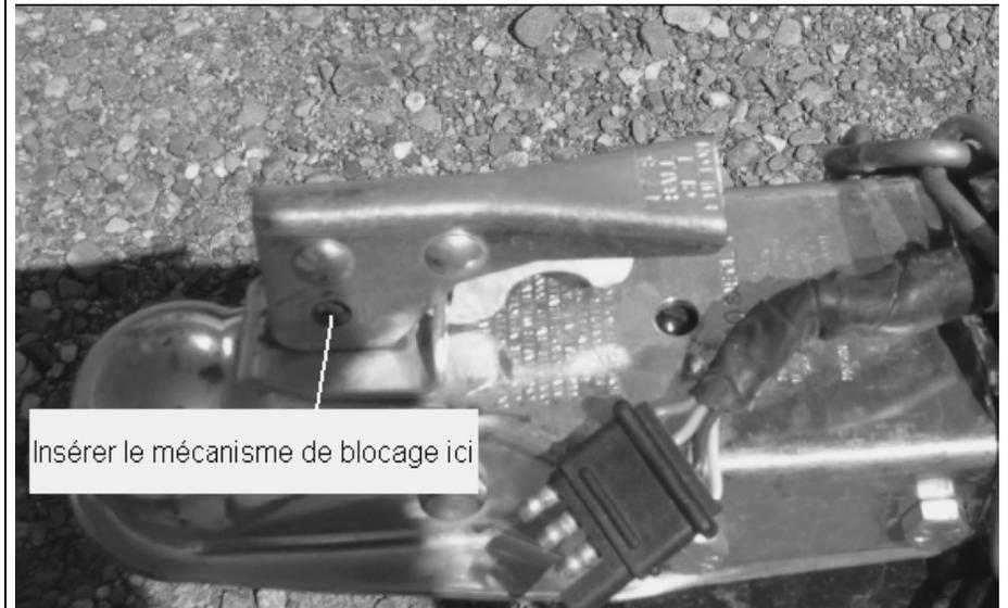
Figure 5.1.2 Insert locking device
