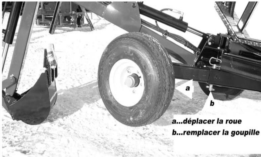
**Figure 5.2.1 (a....move wheel) (b...replace pin)**
