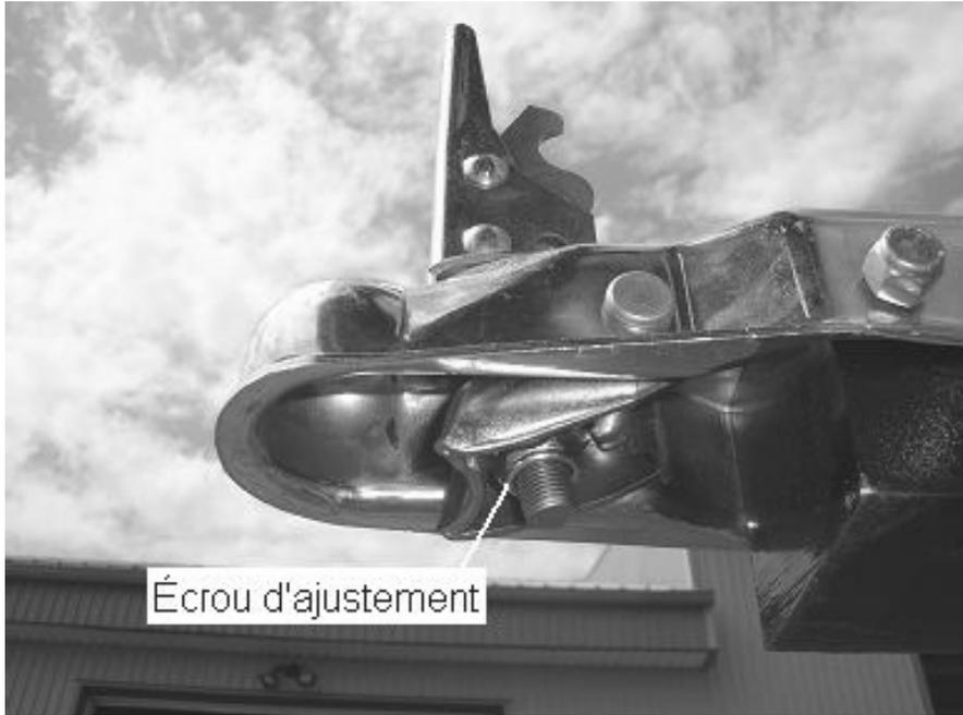
**Figure 5.1.3 Coupler tightening nut**
