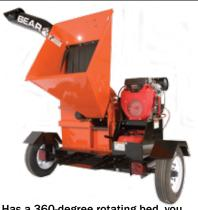
Has a 360-degree rotating bed, you can feed the hopper from any direction. These towable chippers come standard with a torsion axle suspension.
