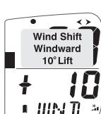
Upwind, wind shift is indicated using a fixed scale of +/- 25 degrees about a central zero. Each segment of the graph corresponds to 2.5 degrees of shift.
