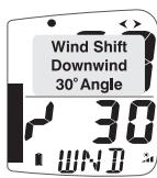
Downwind, the graph indicates the angle sailed relative to the Mean Wind Direction (MWD) from a zero at the bottom of the graph. Each segment of the graph corresponds to 2.5 degrees of shift.
