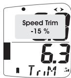
Speed trim is indicated using a default scale of +/- 25 percent about a central zero. The scale can be set between +/- 25 and +/- 100 percent in setup.
