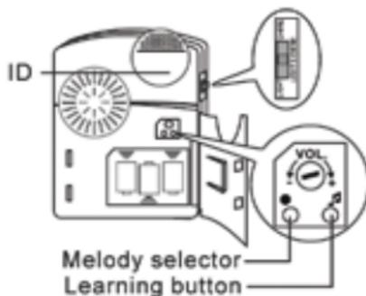
After selecting the zone and melody, press the remote button once (the remote button must be within 3 feet of the chime when programming.) If the coding is successful, the chime will generate a short tone.
