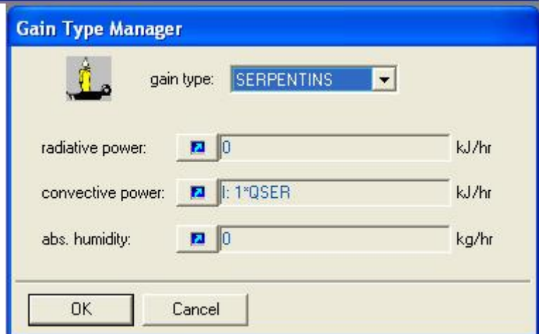
Figure A3.11 Input parameters in BREBID for the definition of the input convective heat gain in the zone PONT
