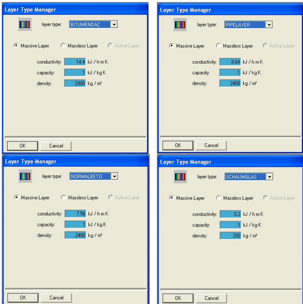
Figure A3.10 Input parameters in BREBID for the thermal characteristics of the various material layers
