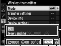
The screenshot shows the 'Wireless transmitter' menu with the following items: Mode, Transfer settings, Device info, Device settings, and PCI. Below the menu, the status display shows 'Now sending DSC\_0001.JPG' with a progress bar, a timer '00:00:00', and a battery icon.
