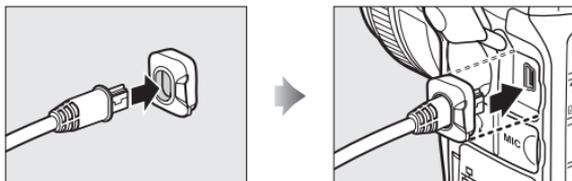
When connecting the USB cable to a D800 or D800E, attach the supplied UF-3 cable cover as shown.
