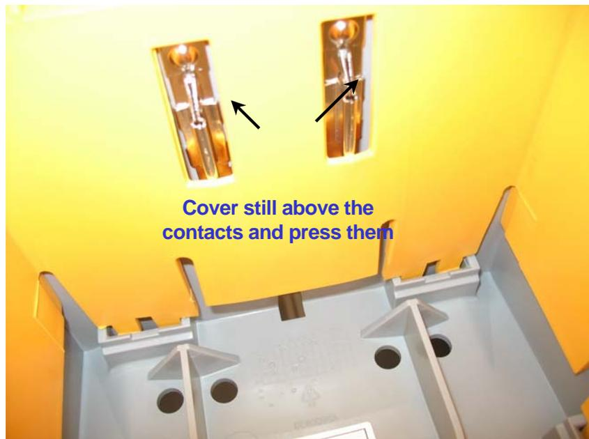
4. Use a rubber or silicon hammer to hit both sides as shown in the pictures below to insert the cover to its place:
