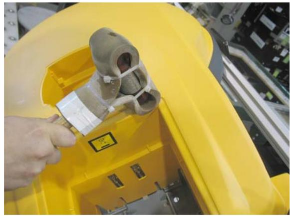
5. Confirm the battery contacts are stick out of the cover and are not free to move.
