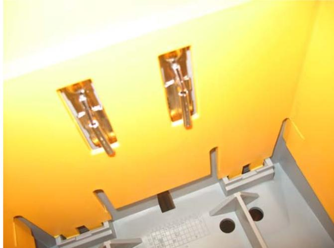
2. If you find it difficult to assemble the cover, then it is possible to simply cut the new rib in the middle and to assemble it as always done.
