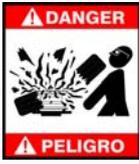
Overinflated tires or tires mounted on the wrong sized rims can explode producing hazardous flying debris.
