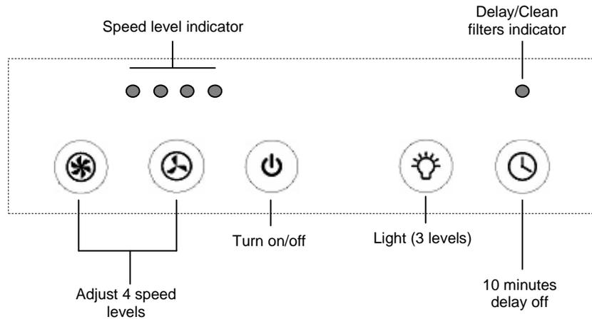
**On/off button:** This button will turn off or on (at speed level 1) the fan.
