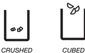
For crushed ice, cubes are crushed before being dispensed. This may cause a slight delay when dispensing crushed ice. Noise from the ice crusher is normal, and pieces of ice may vary in size. When changing from crushed to cubed, a few ounces of crushed ice will be dispensed along with the first cubes.
