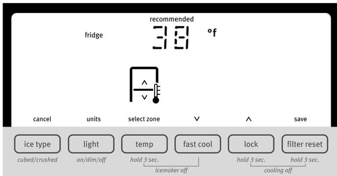
**NOTE:** To view Celsius temperatures, press the LIGHT button when adjust mode is activated. To return the display setting to Fahrenheit, press LIGHT again.
