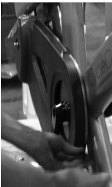
Fig. 1 – Remove chain guard
