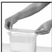
2. Place the filled container into the housing and cover with the housing lid.
