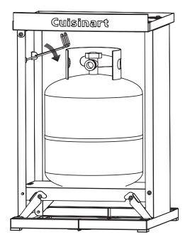
20 lbs LP tank Use: For use only with standard sized 20lbs, LP tanks (approximately 18 1/4" high, 12 1/4" diameter).
