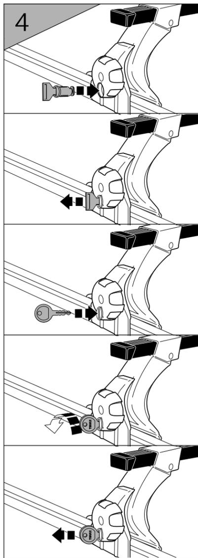
Use the change key to install the lock cylinder. Once the cylinder is installed remove the change key and insert the lock key. Turn the key 180° counter-clockwise to lock, *the knob spins freely in the locked position.*
