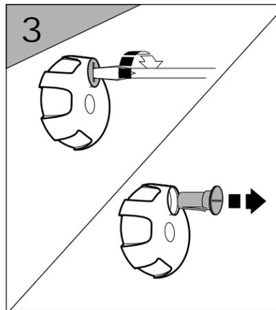
When using lock cylinders you must remove the plug in the locking knob. Using a screwdriver, turn the plug clockwise 1/4 turn, then pull the plug out. If you opt not to use lock cylinders, leave the plug in place.
