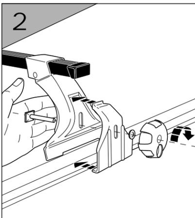
Open the car doors before attaching to the roof. Position the foot behind the car's rain gutter. Attach the bracket around the rain gutter by feeding the bolt through the foot, bracket and washer. Before you begin to tighten with the locking knob, make sure the load bars are positioned evenly in between the feet.
