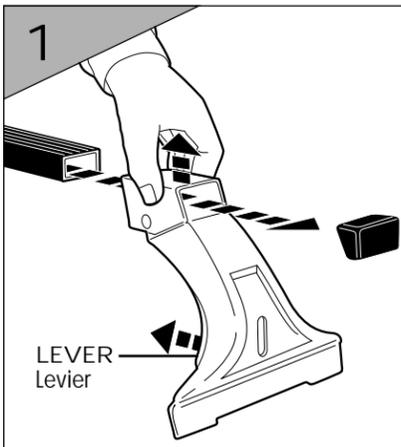
Slide the load bar through the feet. You may need to pivot the top of the foot and pull out the lever to allow the bar to slide through. Attach the end caps to the load bars.
