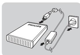
Put the Power Adapter (B) and the Power Cord (C) together and connect them to the external hard disk and a power outlet.
