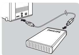
Plug the USB cable (D) in the USB port of your external hard disk. Connect the other side of the USB cable to an empty USB port of your computer.
