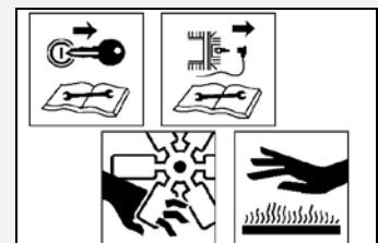
⚠ Take care during maintenance with any moving parts (e.g. pulleys, fans) and with parts subject to high temperatures (e.g. exhaust pipe, engine block, cooling liquids and lubricants).
