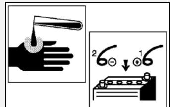
Remove the battery from the machine by disconnecting the poles before proceeding with any battery operations (start-up or fill-up).
