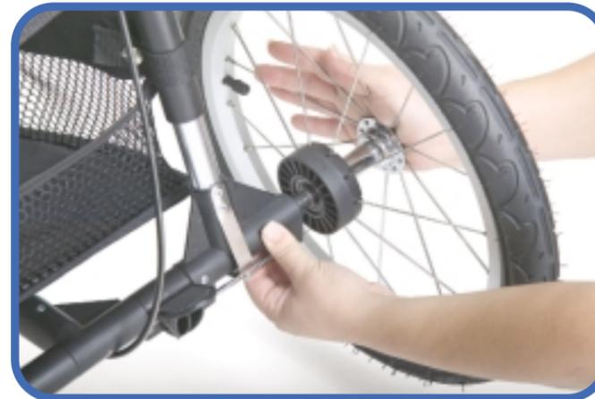
• To remove, simply push in the spring lock while pulling out the wheel.
