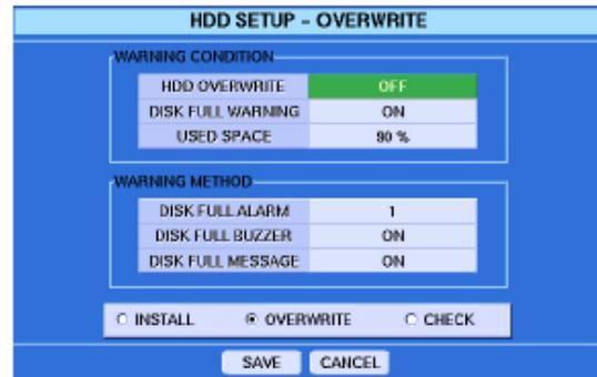
Figure 41 – HDD Setup – OVERWRITE(2)
