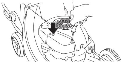
Remove the air filter and check that it is undamaged. Replace with a new air filter if you believe it to be defective.
