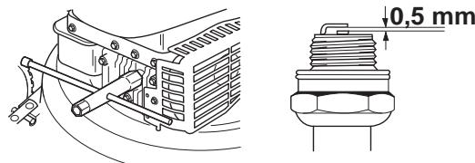
**CAUTION!** Always use the recommended spark plug type! Use of the wrong spark plug can damage the piston/cylinder.
