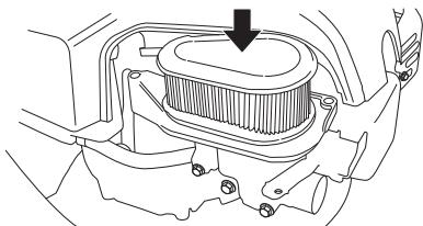
Clean the filter by knocking the filter against a flat surface. Never use solvent with petroleum, for example, kerosene, or compressed air to clean the filter.
