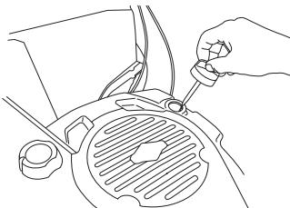
The oil filler cap must be completely screwed down to give a correct picture of the oil level.
