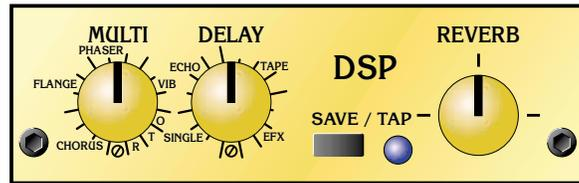
effects is given below. The Multi control selects the “pitch modified” and wah effects. Many of these effects have their speed controlled by the Save/Tap button. The Delay control selects the delay or echo effects. All of these effects have their speed controlled by the Save/Tap button. Additional information is provided on pages 5 and 10.
