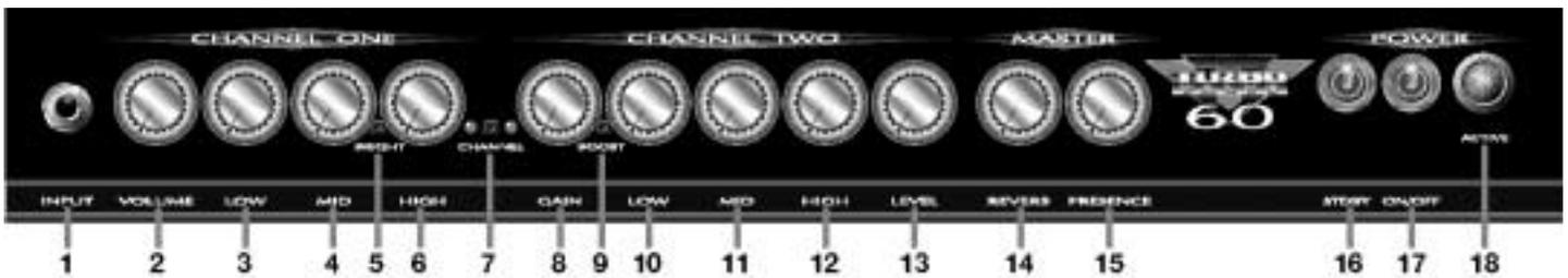
**1. INPUT:** Connect your guitar or wireless receiver into this standard 1/4" jack using a shielded instrument cable.
