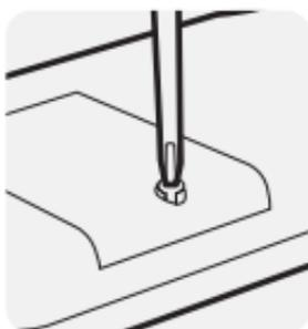
Remove the screw from the battery compartment.
