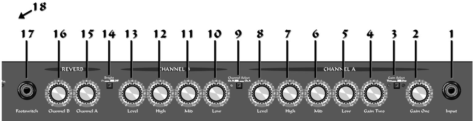
**1. INPUT:** Accepts the mono 1/4" plug of the signal cable from your guitar or wireless receiver.
