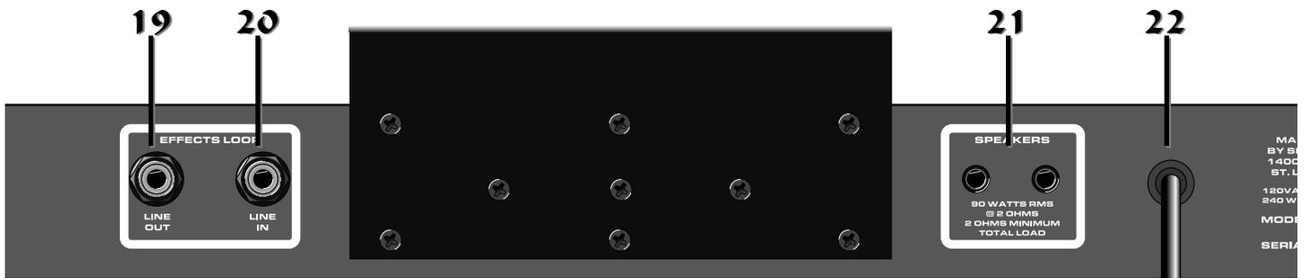
**19. EFFECTS LOOP LINE OUT:** Sends a signal out to your effects devices or signal processors. Lets you add effects, with lowest noise. Uses a shielded signal cable with mono 1/4" plugs. Also doubles as a source for a post-EQ, pre-amp signal to send your signal to a mixing board, recorder, powered monitor or external amplifier.
