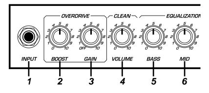
1: INPUT: Connect your guitar here using a shielded instrument cable.
