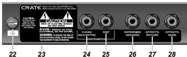
**22: FUSE:** The fuse protects the amplifier from damages caused by a faulty AC power source and/or other problems. If the fuse opens, replace it **ONLY** with the same size and type. If fuses continue to fail, check the AC source – if the source is okay, contact your Crate dealer for service information.
