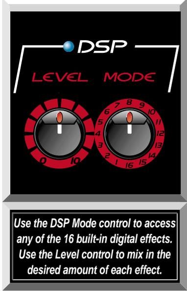
Use the DSP Mode control to access any of the 16 built-in digital effects. Use the Level control to mix in the desired amount of each effect.
