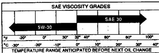
**NOTE:** Although multi-viscosity oils (5W-30, 10W-30, etc.) improve starting in cold weather, these multi-viscosity oils will result in increased oil consumption when used above 32°F (0°C). Check your engine oil level more frequently to avoid possible engine damage from running low on oil.
