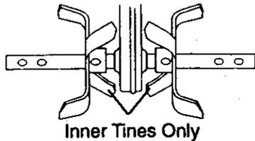
**NOTE:** When reassembling outer tines, be sure right tine assembly (marked "R") and left tine assembly (marked "L") are mounted to correct side of tine shaft.
