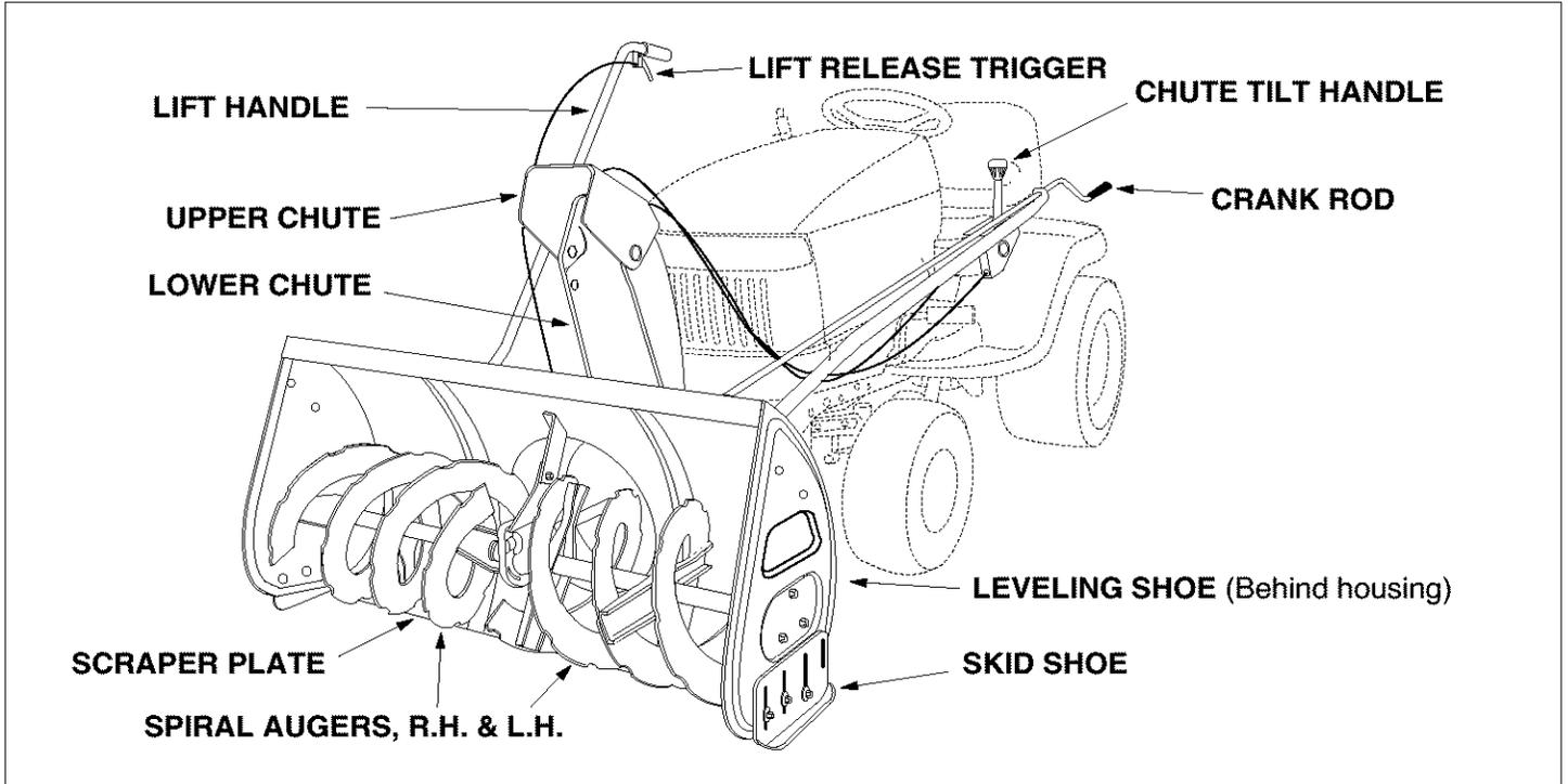
**CHUTE TILT HANDLE** Pivots the Upper Chute up or down to control the angle and distance of discharge.
