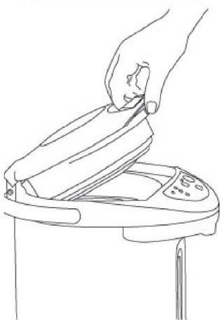
\*Pull the latch of lid lock upward, and then open the lid.
