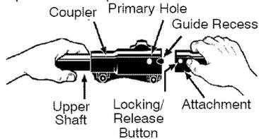
3. Push the attachment into the coupler until the locking/release button snaps into the primary hole.
