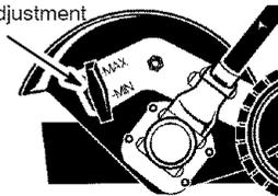
1. Loosen the depth adjustment knob.
