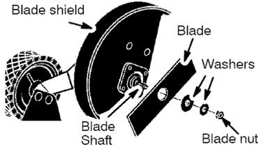
5. Install new blade onto blade shaft.
