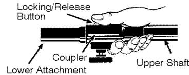
3. While securely holding the upper shaft, pull the attachment straight out of the coupler.
