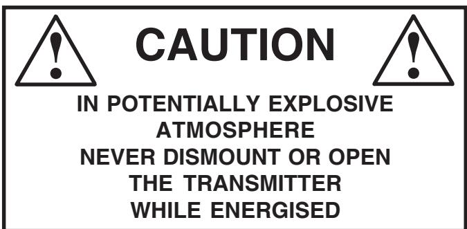
*The above instruction applies only to the "flameproof enclosure" protection mode (EEx "d" equipment as described in § 2.2). It is not applicable to the other protection modes EEx "ia", EEx "nAL" and EEx "nL" as described in § 2.1 and § 2.3.*
