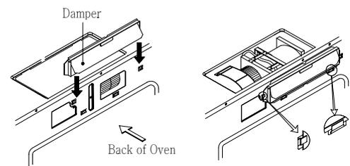
After adjust the damper, reinstall the blower motor cover with the screw (①).
