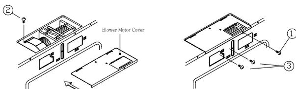
Carefully match the exhaust opening location of the microwave and attach the damper to blower motor cover by sliding it into the guides at the blower motor cover.
