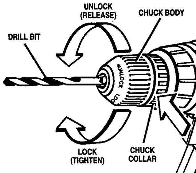
**WARNING:** Do not hold chuck body with one hand and use power of the drill to tighten chuck jaws on drill bits. Chuck body could slip in your hand or your hand could slip and come in contact with rotating drill bit. This could cause an accident resulting in serious personal injury.
