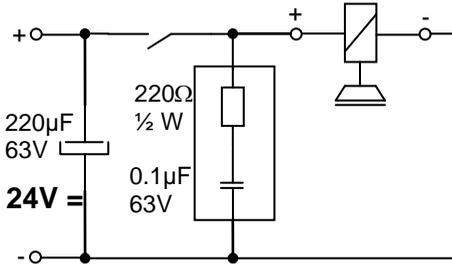
In a servomotor with brake, check that it works before running the motor. The standard brake has a 24 V ± 10 % DC supply. Servomotor brakes should not be used to stop the motor but to immobilize it in rotation when it is stationary. The holding brake is used for many repetitive dynamic brakings but the dynamic braking is only reserved for emergency stop.
