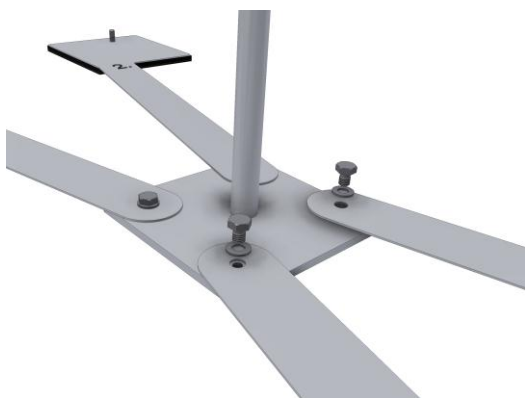
Fig. 3: Bolting the feet
