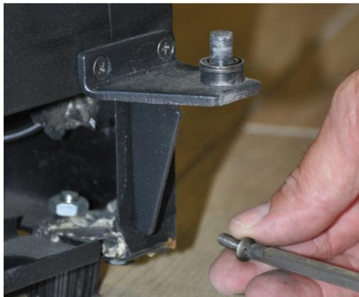
Remove the bottom pivot. Keep all components for later use, as shown in Step 10.
