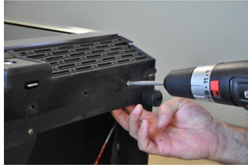
**Reinstall the vent grid using the 10 screws.**
