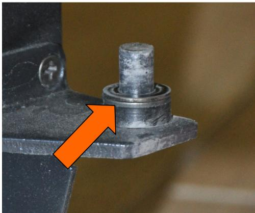
Keep the leveling rings for later use as shown in Step 10.
