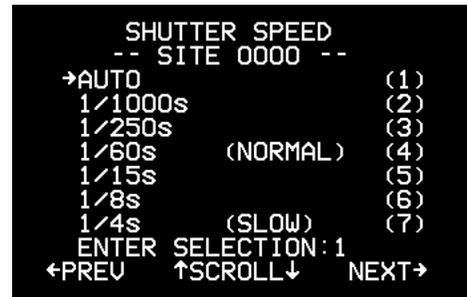
Figure 34. Menu Shutter speed (Vitesse d'obturation) (PAL)
