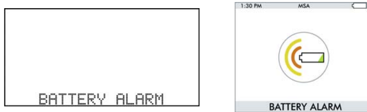
Figure 2-5. Battery Shut Down
