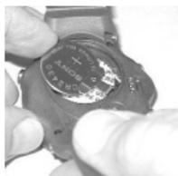
Fig. 70 - INSTALLATION DE LA PILE
