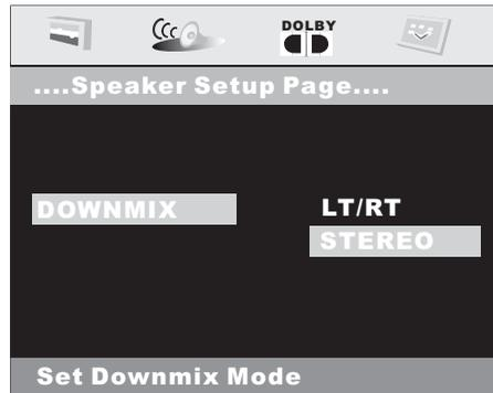
This is to activate the audio output from DOLBY AC3 5.1 DOWNMIX to 2 channel mode. Select the preferred SPEAKER connection by using the cursor buttons. Select the LT/RT to activate the Dolby surround compatible output. Select the STEREO to activate simple stereo mode.
