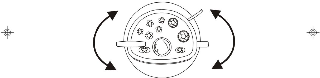
**FM** – The FM antenna is built in to the AC power cord. If FM reception is weak try varying the position and direction of the power cord until you find the strongest signal.
