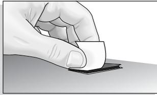
4. Attach the detector to the hook-and-loop fastener. You can remove and reattach the unit as often as you like.
