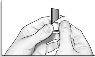
3. Attach the pad to the dashboard at your chosen location and remove the other paper backing.
