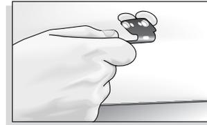
3. Push the bracket firmly onto the windshield.
